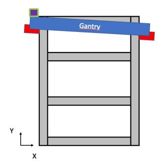
At the moment when the gantry reaches the limit switch, both stepper motors stop, but the gantry is still not squared. This is where Gantry Squaring comes into play, and it can be extended with this extension board if the control system does not support Gantry Squaring on its own.
