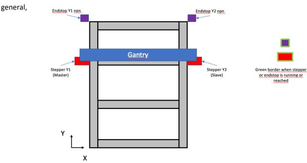
depending on the mechanical design, the gantry is aligned at a right angle. However, it might be possible that the gantry is not at a right angle due to the construction of the milling machine or its stability. In such cases, it is indeed possible for a gantry to be misaligned (exaggerated for illustration purposes).
