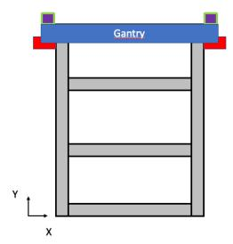
When the second stepper motor reaches the second limit switch, the gantry is squared, and the Gantry Squaring Board forwards the limit switch signal from the master to the control system.
