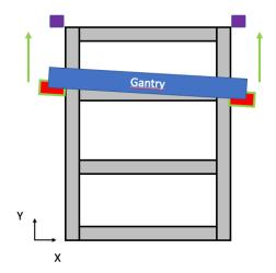
During homing, the gantry initially moves towards the limit switches as usual, with both drives moving towards their respective limit switches.
